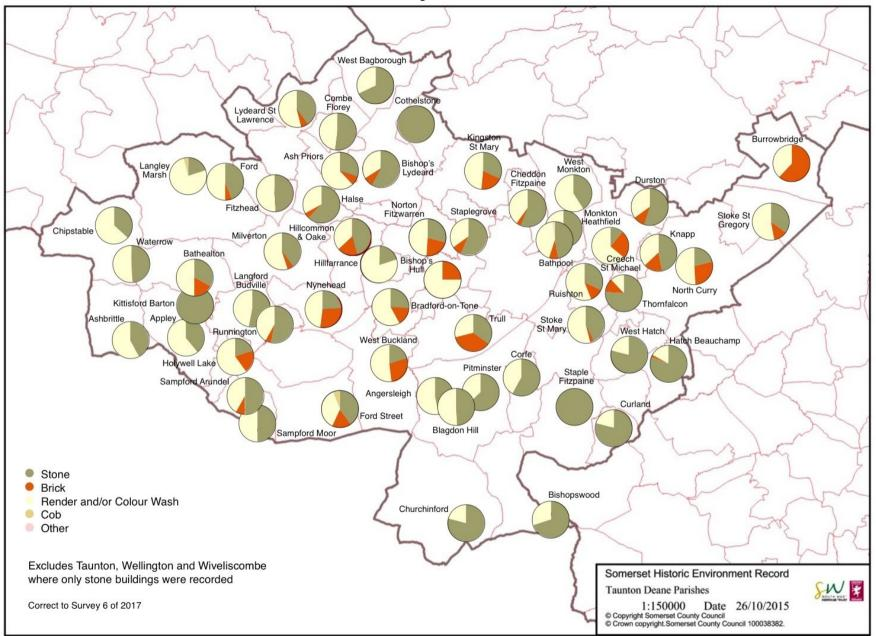
Materials used in the construction of the external walls of buildings
