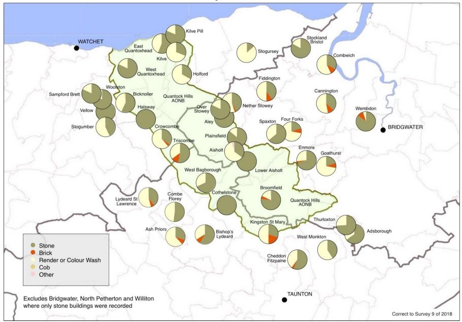
Materials used in the construction of the external walls of buildings
