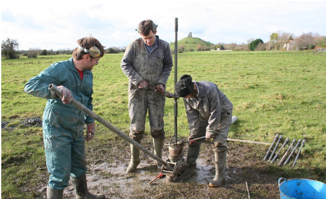
The extraction of a percussion core at Southlake Moor.
