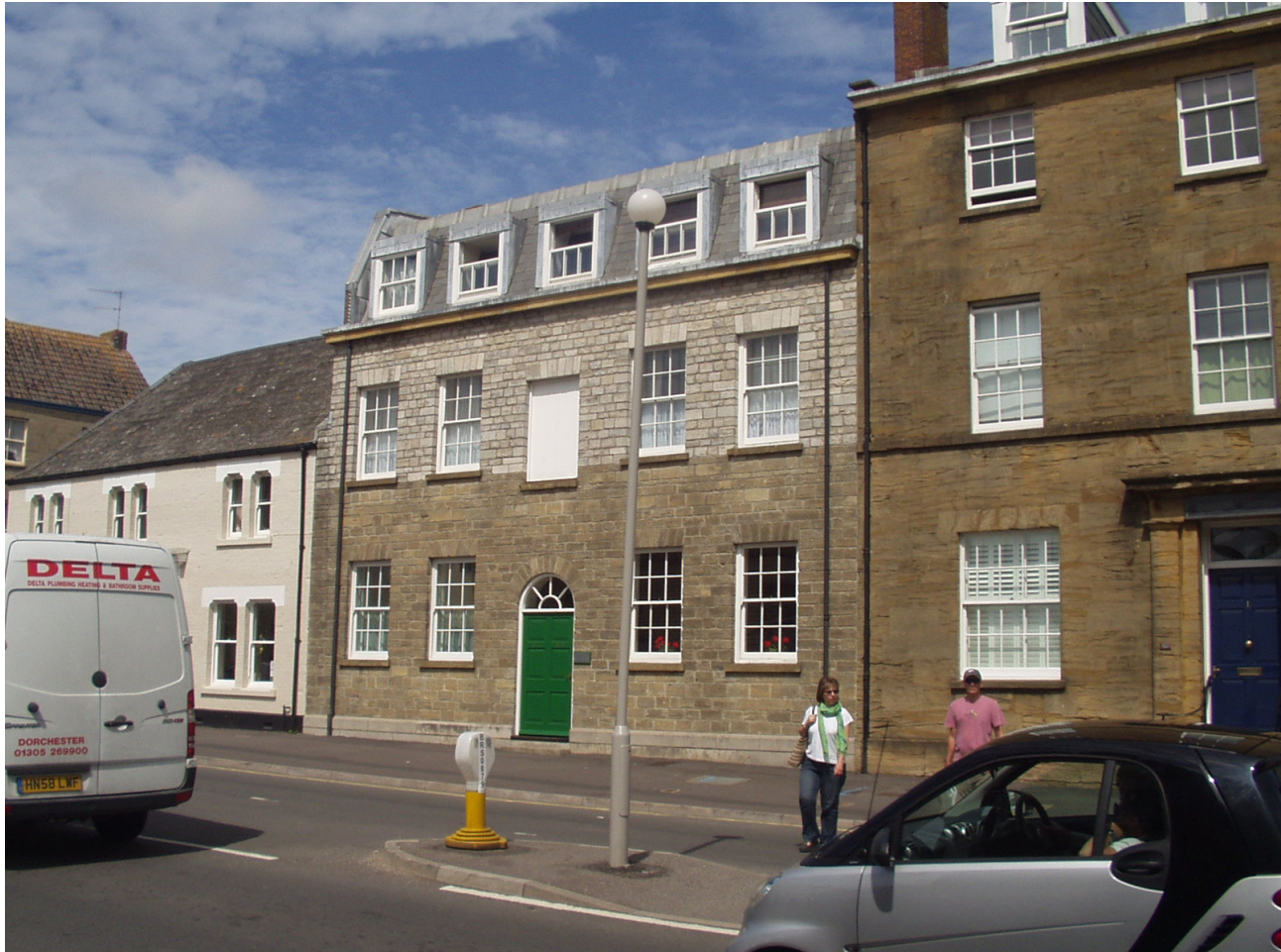
Figure 5. Stevenson Court, 61 East Street, Bridport. The ground floor is finished in locally won Forest Marble, the first floor in imported stone of Code 64. The building on the right is finished in Ham Hill Stone.
