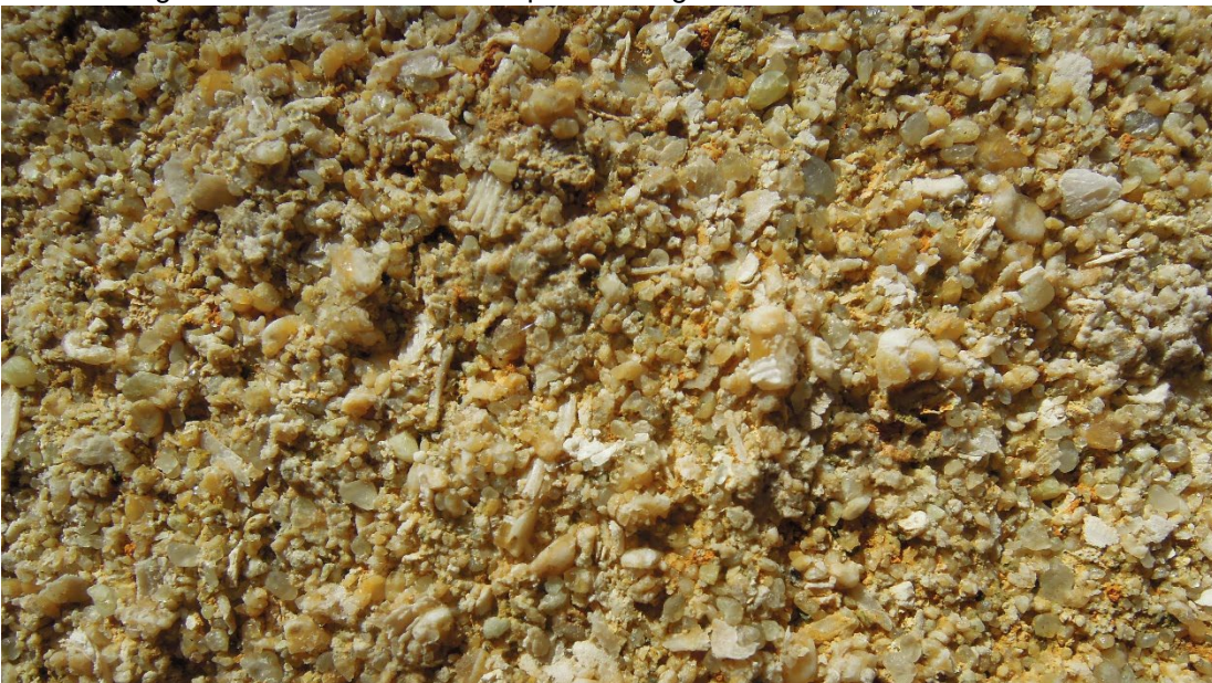
Figure 4. Texture of Salcombe Stone showing poorly sorted clasts of both quartz and calcite, including shell fragments. St Francis' church, Woolbrook, Sidmouth. Width of photo. 2cm.
