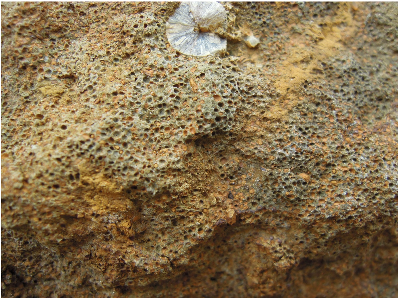
Figure 1. Ochre oolitic limestone, garden wall, Farthings, Abbey Street, Hinton St George. Width of crinoid ossicle, about 5mm.
