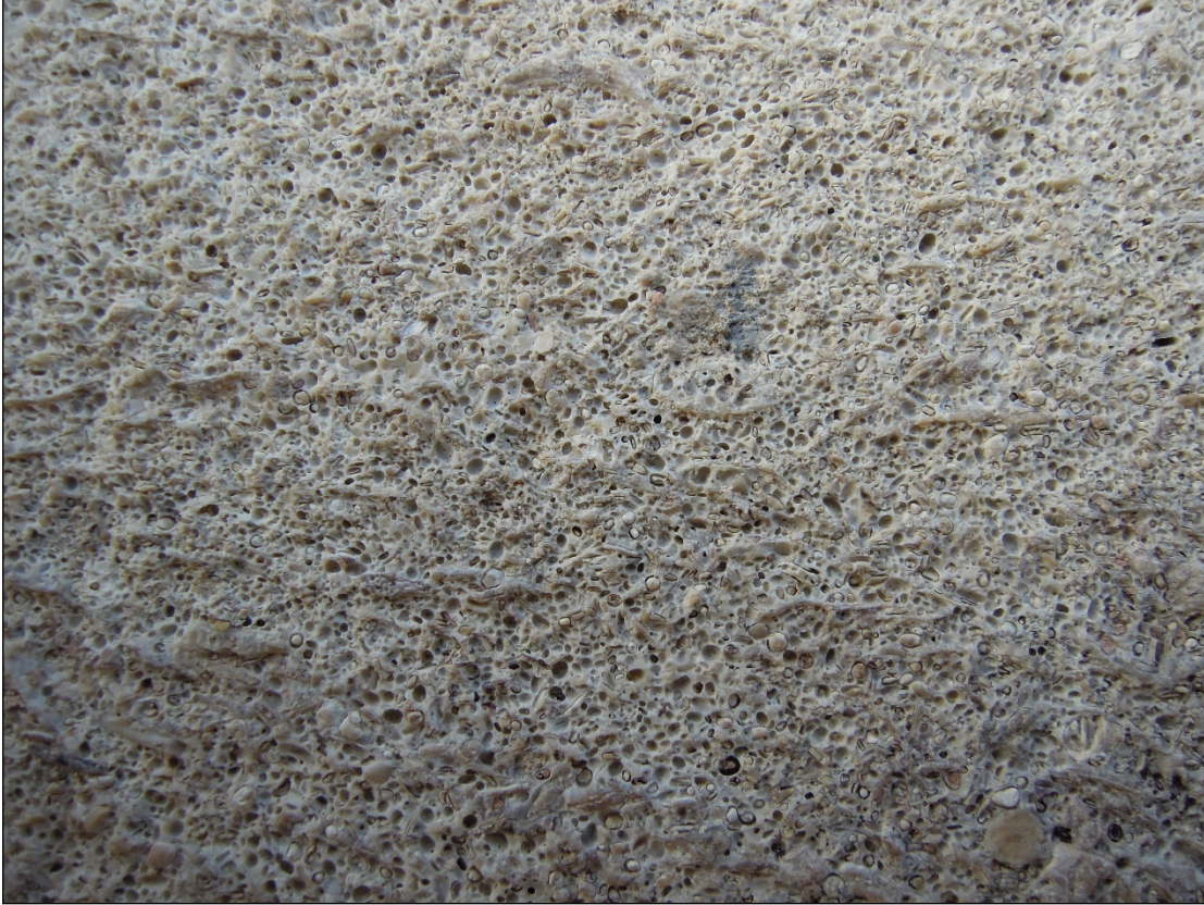
Figure 6. Booking Hall, railway station, Axminster. Oolites are about 1mm across. Aligned shell fragments define a crude bedding fabric in this example but are not always present.
