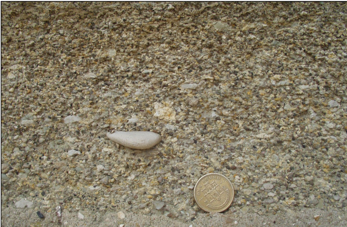
Figure 6. Tower of All Saints church, Norton Fitzwarren. Very coarse-grained sandstone composed of quartz, hard dark exotic rock-types and intraformational clasts of pale grey calcareous siltstone.
