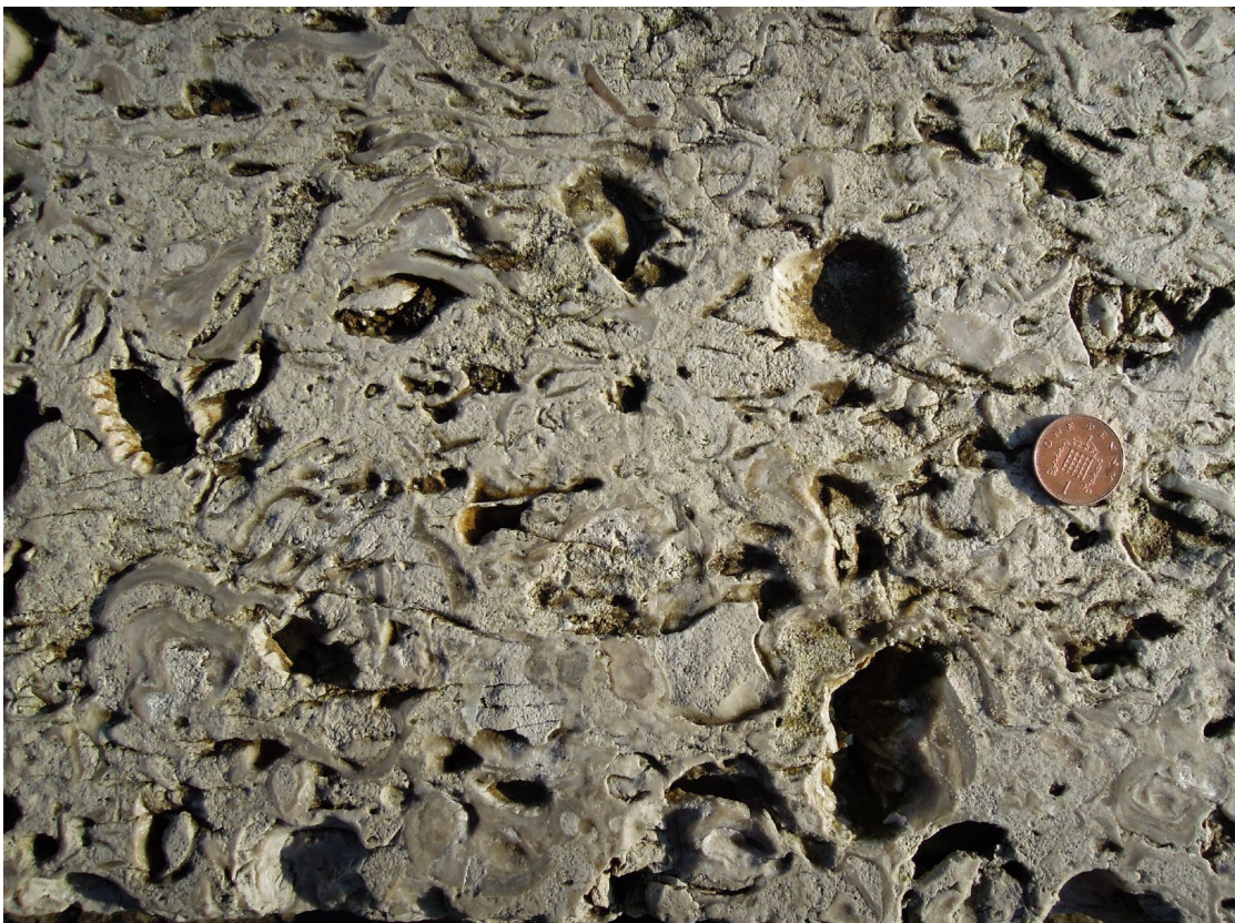
Figure 1. Negative casts of bivalves and gastropods in Portland Roach used for the facing of the Cob, Lyme Regis.
