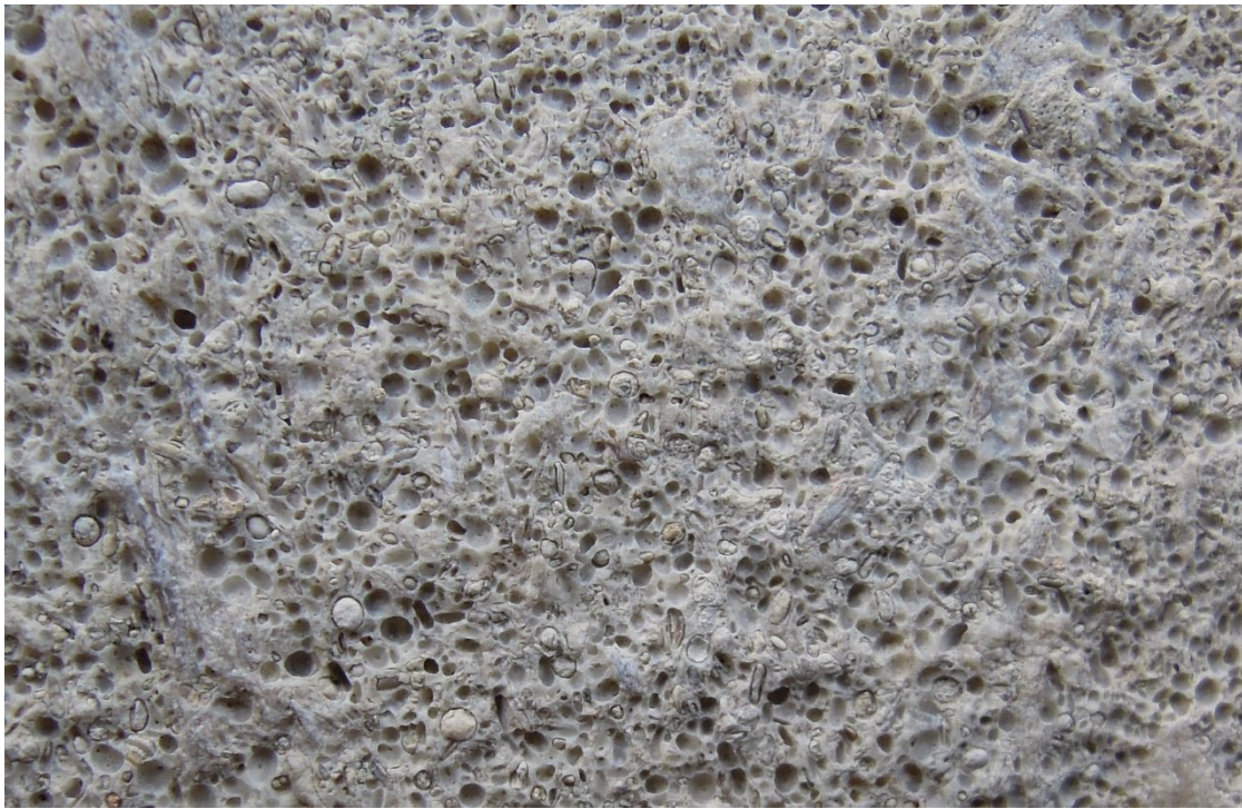
Figure 7. Detail of the photo above. The rock typically breaks round the oolites, most of which fall out of the exposed surface.
